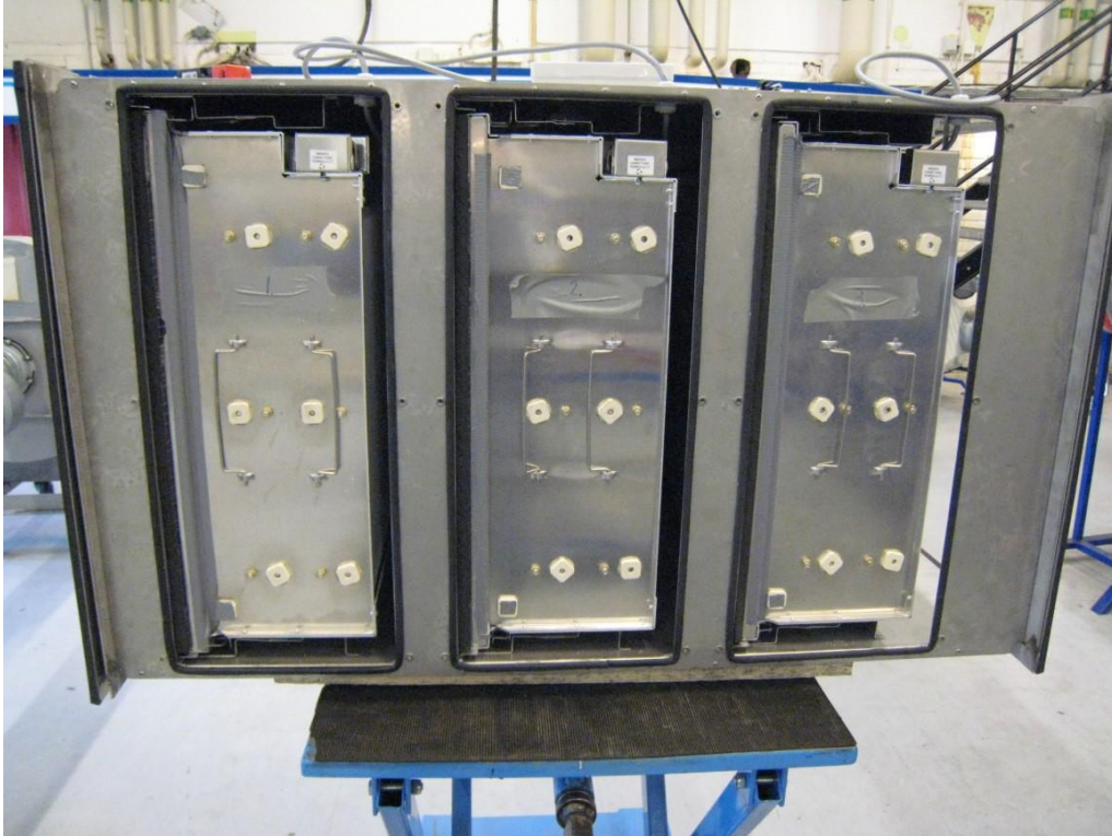
Fig 5. Three FE600 mounted in series in the duct section, side view
